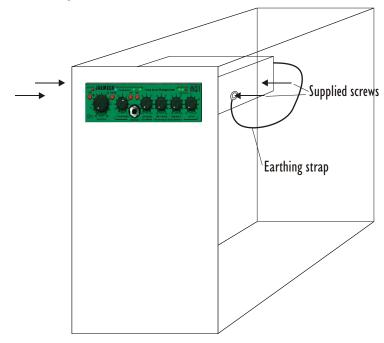
Make sure that the earthing tag has a good metal-metal connection to the computer case. This ensures maximum noise performance when recording.
