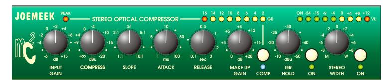
INPUT GAIN – sets the amount of audio amplification. Too little gain and the resulting sound will be too quiet; too much and the signal could become distorted.
